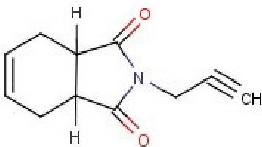
$^1\text{H}$ - NMR (DMSO- d6):  $\delta$ , 3.15(s, 1H), 4.05(s, 1H,  $\text{CH}_2\text{-C}$ ), 5.90 (s, 2H,  $\text{CH}=\text{CH}$ ), (Fig 3.1).
